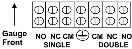
The terminal strip will accept wires in the range of 22 Awg - 16 Awg.. Reinstall the cover, and (4) screws after connection of field wiring.
