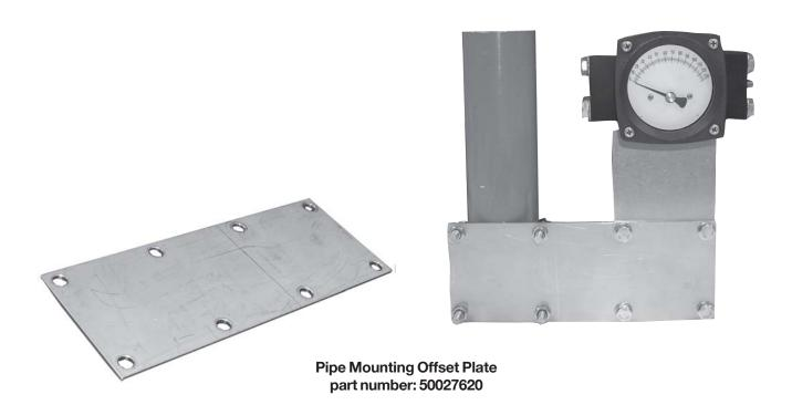
Used to hold pipe mounting bracket away from pipe in order to access rear gauge connections.
