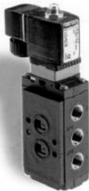
3/2-way valve with exhaust recycling, in de-energized position, port 2 feed back internally
