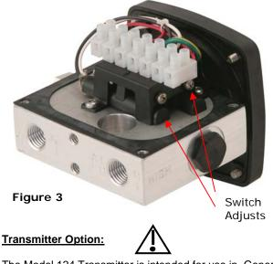
The Model 124 Transmitter is intended for use in General Purpose Locations. This enclosure carries\_a NEMA 4X environmental rating.
