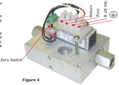
The weather-proof enclosure comes standard with a  $\frac{1}{2}$ " FNPT conduit interface. Internal to the enclosure is a 4 position terminal strip. The terminal strip accepts wire sizes 22 AWG – 16 AWG. Connections are defined in Figure 4.
